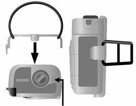
Secure PLB1 using lanyard attachment
